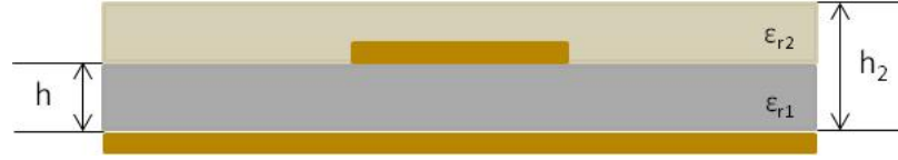
Figure 2.2: Microstrip with Dielectric Overlay
